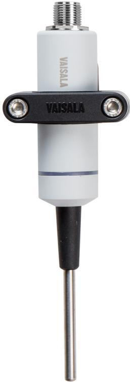
Vaisala HUMICAP® Humidity and Temperature Probe HMP1 is designed for ambient measurement in indoor spaces. Its probe head and body are integrated into a single unit with no cable between them. HMP1 can be directly connected to Indigo200 series transmitters to form a single wall-mounted unit.
