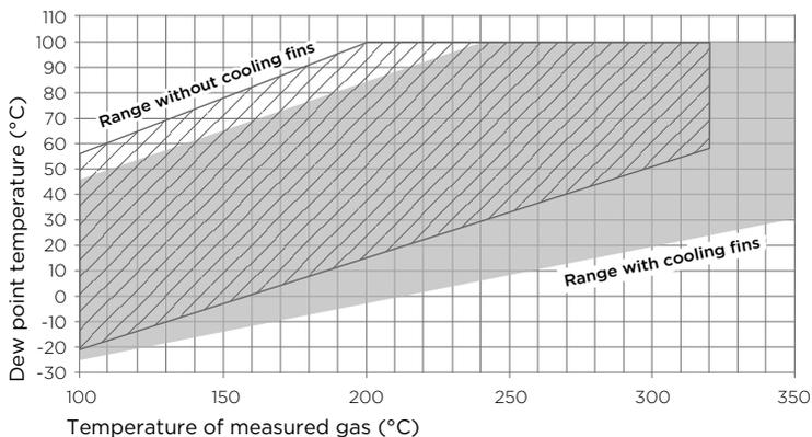
Figure 7 Operating range of DMP6 probe head
