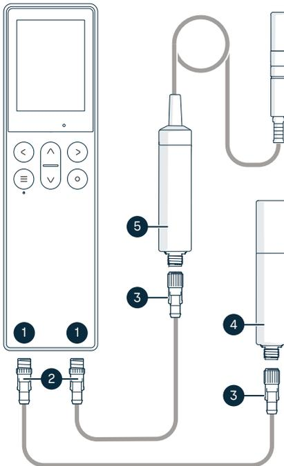
Figure 21 Example of connecting probes to Indigo80
