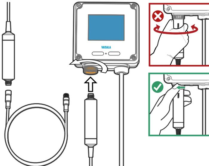
Figure 17 Connecting probe to Indigo200 series transmitter
