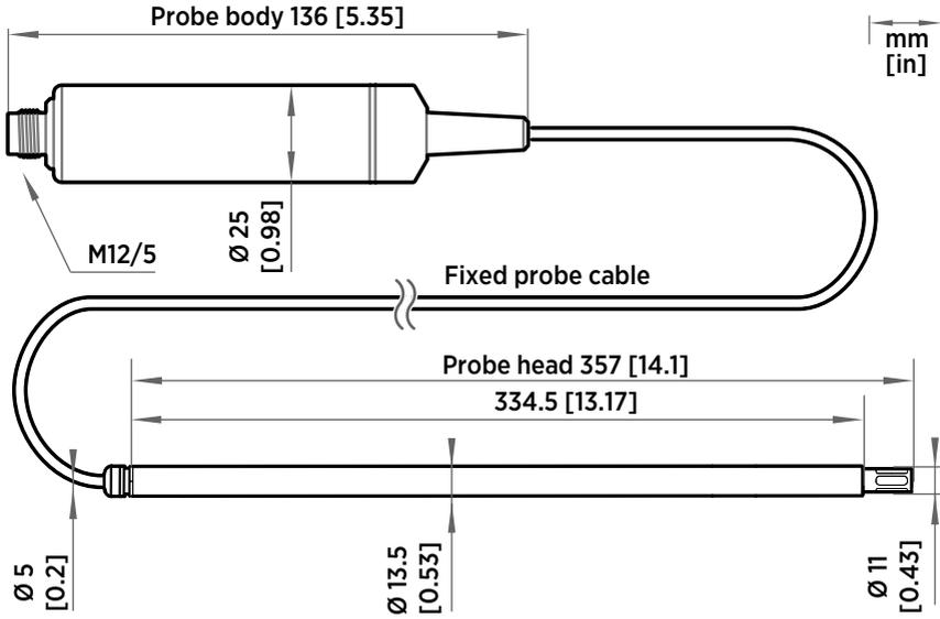
Figure 5 DMP6 probe dimensions
